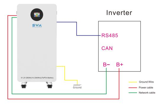
Step 1.If multiple batteries are used in parallel, manually press the low-voltage switch (ON/OFF) first. Use a multimeter to check if the voltage of each battery is consistent. If consistent, turn off the batteries and proceed with cable connections, as shown in the schematic diagram (using two batteries in parallel as an example).
